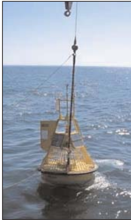
3-meter buoy on station. The vertical bars around the deck of the buoy are called "seal cages" and are placed on buoys to prevent seals from climbing aboard, thus avoiding possible harm to the seal while preventing damage to the buoy.
