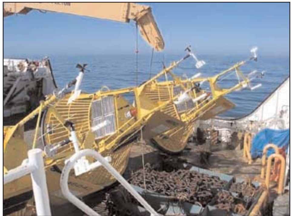
3-meter discus buoys in a diagonal position along the deck with the Aspen's crane poised overhead.
