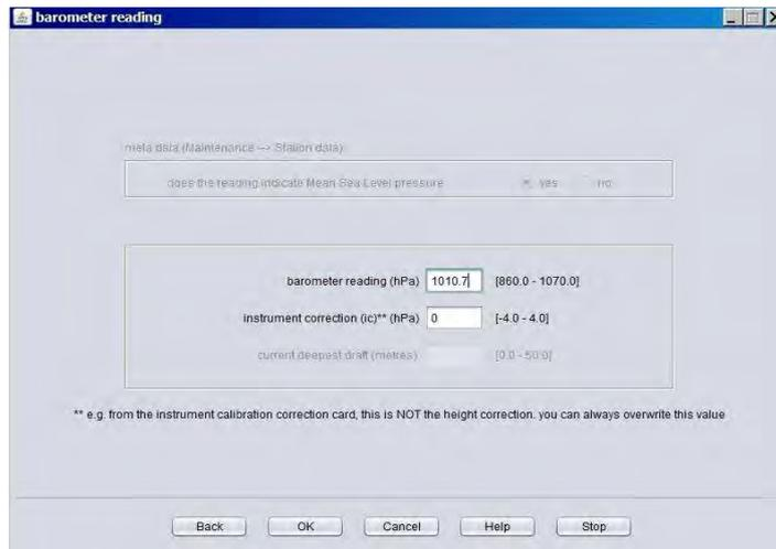
Figure 6: Barometer Reading
